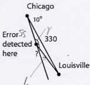
$$a) \text{ Speed} \cdot \text{time} = 220 \text{ mph} \cdot \frac{1}{4} \text{ hr} = 55 \text{ mi}$$
