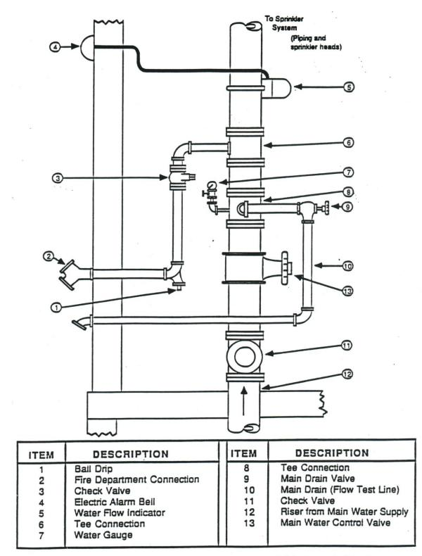
Wet pipe sprinkler system: typical riser with water indicator.
